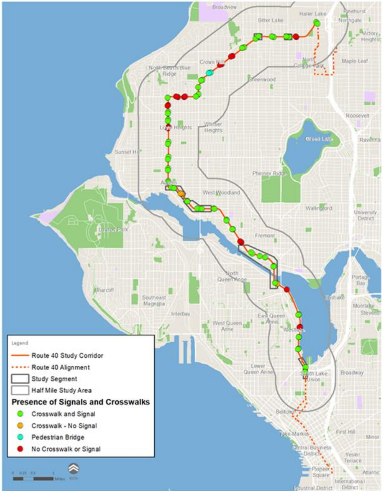
Figure 3: Presence of Signals and Crosswalks throughout the Route 40 Study Corridor Source: SDOT
