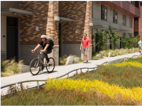
This swale provides for stormwater runoff and enhances the streetscape in the Cascade neighborhood.
